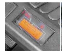
Newly-developed LCD instrument has more comprehensive functions and more stable performance and entirely displays the full vehicle running state, trouble diagnosis and other important information, which can make the operator more intuitively and conveniently have
