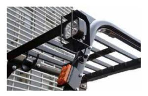
The whole truck adopts LED lights as shiner and new-type panoramic retroreflector to ensure energy conservation and power saving as well as greatly improve the performance and service life of luminaires at the same time.
